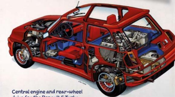
Central engine and rear-wheel drive for the Renault 5 Turbo.
