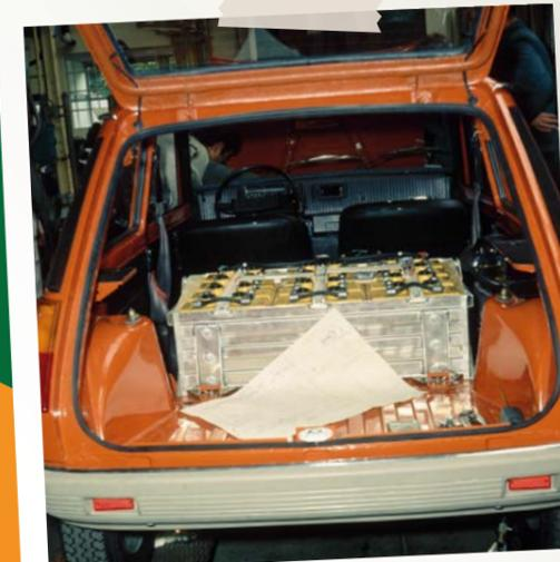
Beneath the rear seat there are 34 batteries.
