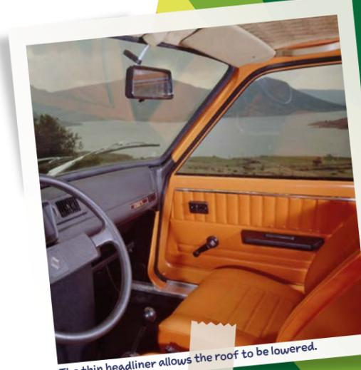
The thin headliner allows the roof to be lowered.
