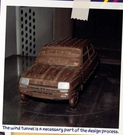
The wind tunnel is a necessary part of the design process.
